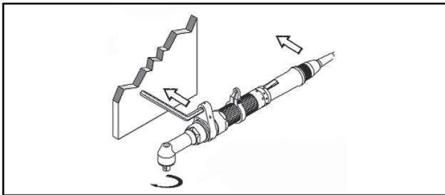
Fig. 7-1: Fixing the reaction bar
