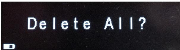
A second press of the delete button will allow you to delete all readings in the list in one go. Just press the green OK button.
