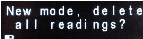
The other time you are forced to delete all readings is when you change the measurement mode mid-way through readings you have already done.
