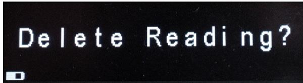
Readings are taken in order, so the first is 1 the last reading would be 999. One press of the delete icon will allow you to delete the *last* reading only. Press the green OK button to do so.
