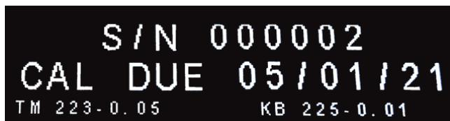
It confirms the serial number of the Torque Analyser you have and its calibration due date. TM is the latest software version of the torque module and KB represents the latest version of the keyboard.
