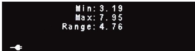
Pressing the up and down arrow keys takes you to the second screen which displays the current minimum and maximum readings as well as the range between them.
