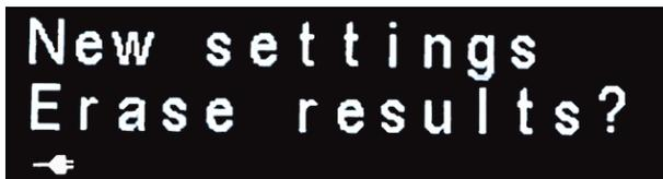
In addition, readings are also deleted when the torque limit specifications are altered.
