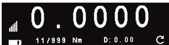
Screen 4 on the fourth press pulse mode with peak value and cycle duration displayed
