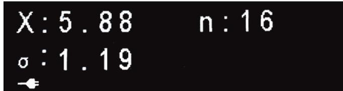
The first screen displays X = Mean average n = Sample count and σ = Sigma (Standard deviation).
